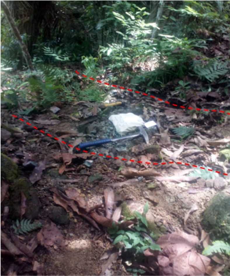
Photo of sampled zone. The width of the zone with visible copper oxides is 0.8m.
