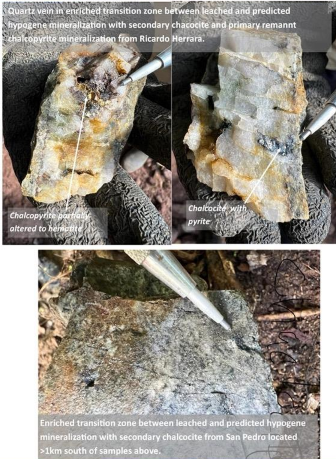
Figure 6. Photos of secondary enriched transition zone with chalcocite and hematite after chalcopyrite.
