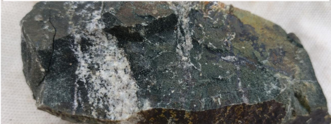
Figure 4. Results initial prospecting at the Sortilegio Porphyry Target at Belen. Handsample from the the boulder 16208 sample of A type vein with pervasive potassic alteration (secondary biotite) and intermediate argillic alteration (chlorite-magneite) disseminated chalcopyrite, with traces of bornite and chalcocite.
